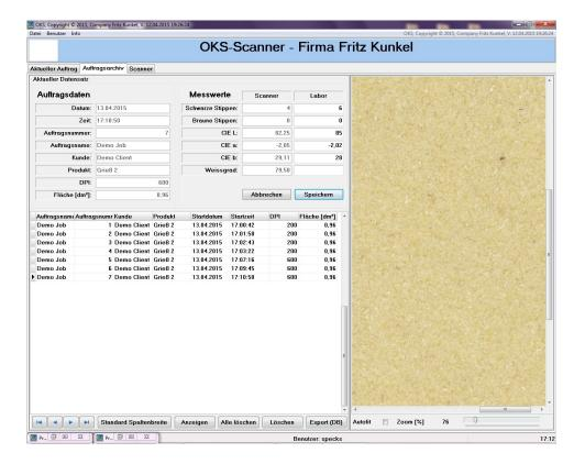
With *OKS scanner*, bulk goods such as flour and semolina, are examined for color, brightness and impurities.
